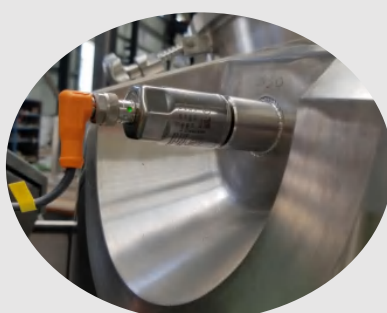
Foaming sensor for control the burner working condition
