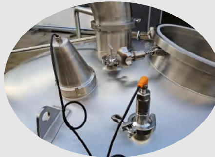
Use for preventing over boiling in kettle tank
