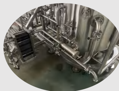
Use for Two-stage wort cooling from Brewhouse to FV
