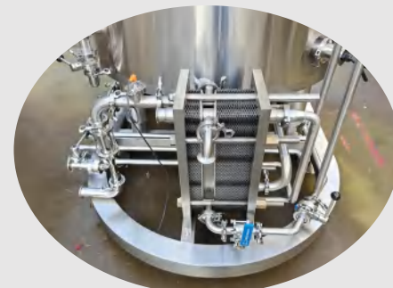
Two-stage PHE for wort cooling during knock-out
