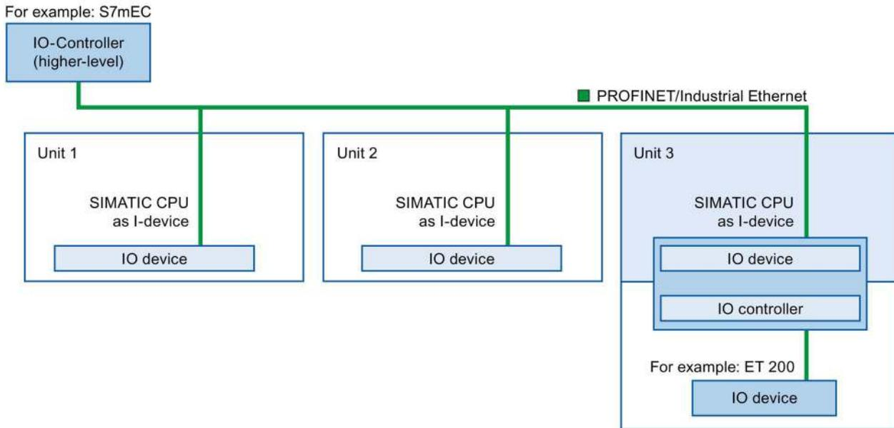
Unit 1 and unit 2 each consist of an I-device with centralized I/O. The I-device along with the distributed I/O system (for example, ET 200) forms unit 3.
