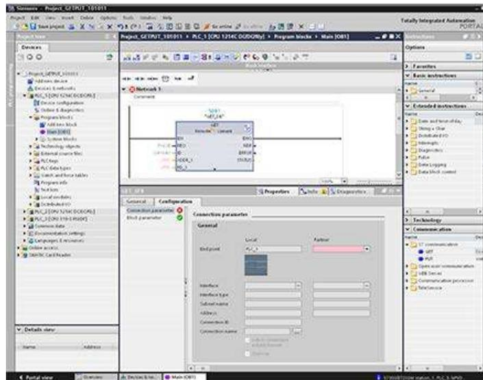
The inspector window displays the properties of the connection whenever you have selected any part of the instruction. You can configure the communication parameters in the "Configuration" tab of the "Properties" for the communication instruction.
