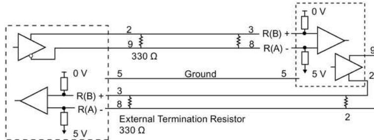
**Case 2: RS422 No cable break detection, forward bias**
