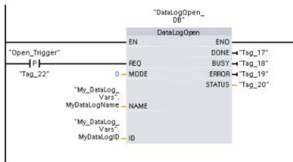
**Network 8** The ID parameter is an IN/OUT type. First, you supply the ID value of the existing Data log whose structure you want to copy. After the DataLogNewFile operation is complete, a new and unique ID value for the new Data log is written back to the ID reference location. The required DONE bit = TRUE capture is not shown, refer to networks 1, 2, and 4 for an example of DONE bit logic.
