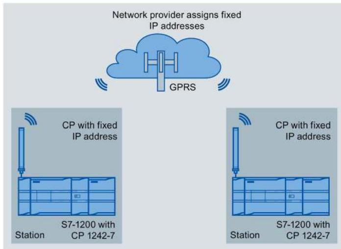
Figure 13-2 Direct communication between two S7-1200 stations
