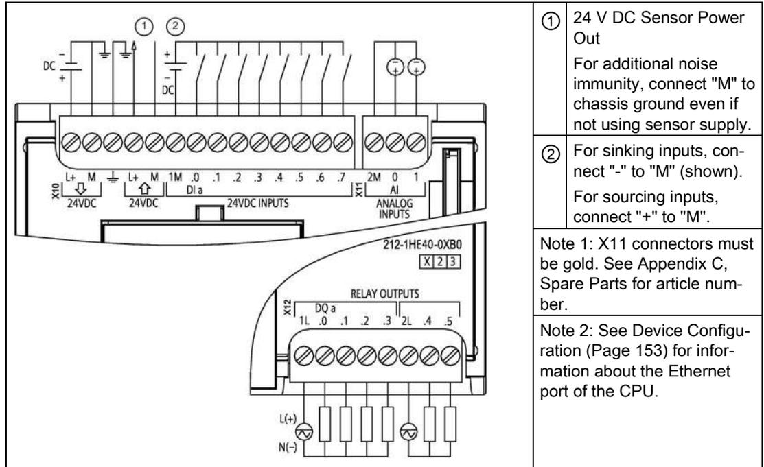
Table A- 44 Connector pin locations for CPU 1212C DC/DC/Relay (6ES7212-1HE40-0XB0)
