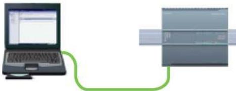
A CPU can communicate with a STEP 7 programming device on a network.
