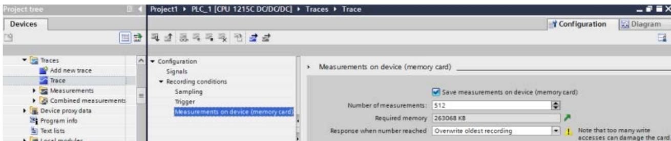
The CPU supports a maximum of 999 trace measurement results. During the time that the CPU is saving the trace measurements to load memory, the CPU does not check the trigger condition for the trace job. Once the CPU finishes saving the trace measurements, the CPU resumes checking for trigger conditions.
