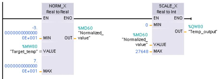
Note that if the analog output was for an analog signal module or signal board using voltage, the MIN value for the SCALE\_X instruction would be -27648 instead of 0.
