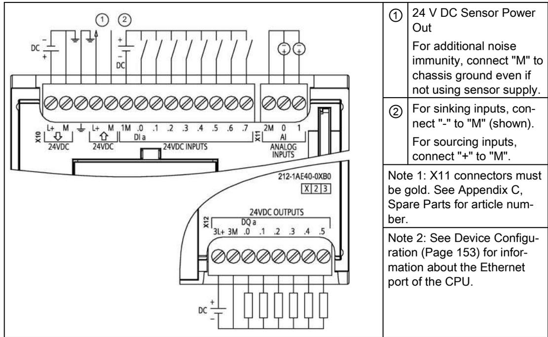
Table A- 46 Connector pin locations for CPU 1212C DC/DC/DC (6ES7212-1AE40-0XB0)
