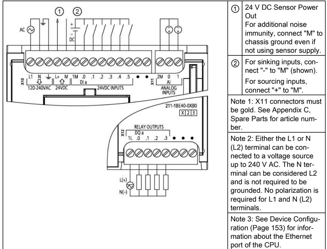
Table A- 23 Connector pin locations for CPU 1211C AC/DC/Relay (6ES7211-1BE40-0XB0)
