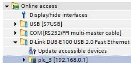
4. From the Online menu of STEP 7, select the "Upload device as new station (hardware and software)" menu command.
