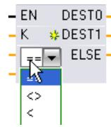
Click a comparison operator inside the box and select a new operator from the drop-down list.
