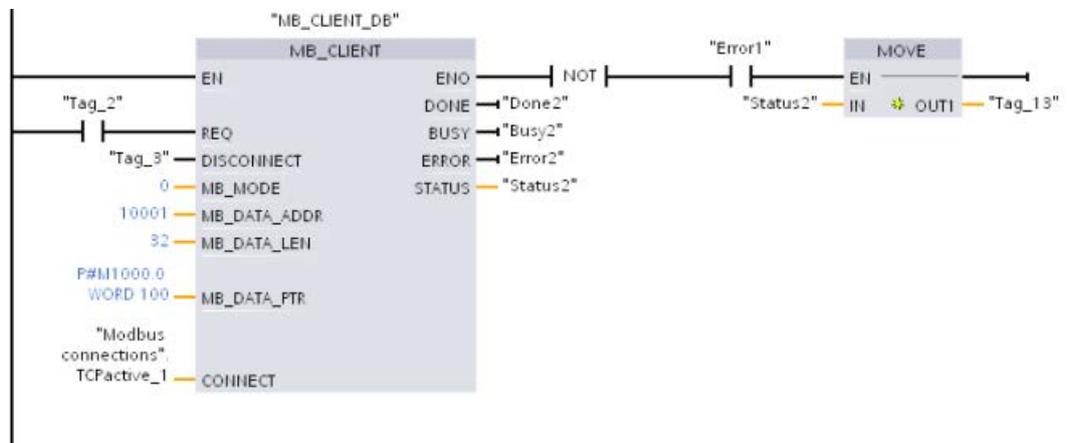
**Example: MB\_CLIENT 2: Multiple requests with different TCP connections**
