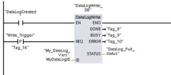
**Network 6** Close the data log once the last record has been written. After executing the DataLogWrite operation that writes the last record, the log file full status is signaled when DataLogWrite STATUS output = 1.
