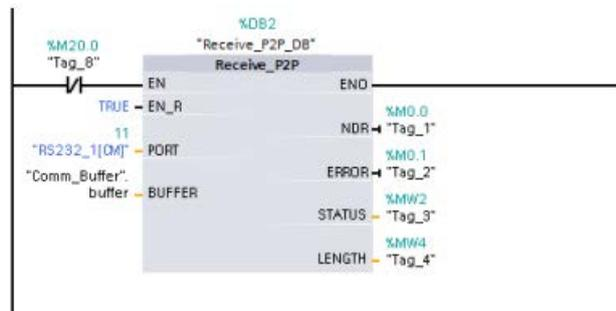
**Network 2:** Use the NDR value (Tag\_1 at M0.0) set by the RCV\_PTP instruction to make a copy of the number of bytes received and to set a flag (Tag\_8 at M20.0) to trigger the SEND\_PTP instruction.
