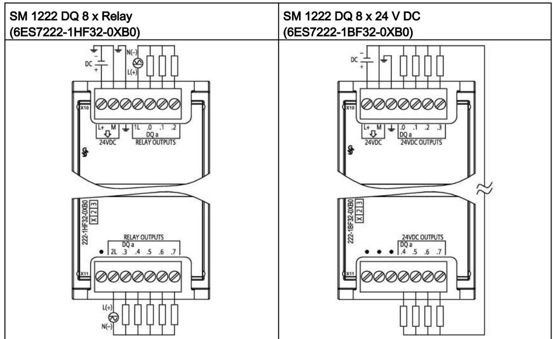
Table A- 116 Connector pin locations for SM 1222 DQ 8 x Relay (6ES7222-1HF32-0XB0)
