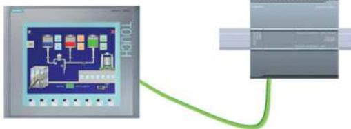
HMI connected to the CPU
