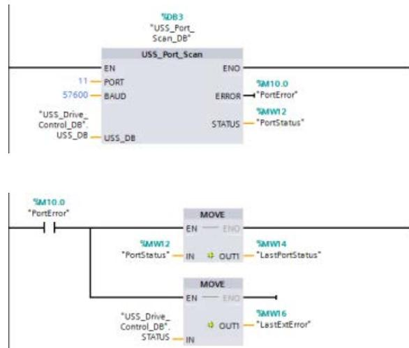
**Network 1** "PortStatus" port status and "USS\_Drive\_Control\_DB".USS\_Extended\_Error extended error code values are only valid for one program scan. The values must be captured for later processing.
