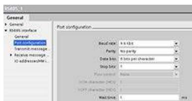
The "Properties" tab of the inspector window displays the parameters of the selected CM or CB. Select "Port configuration" to edit the following parameters:
