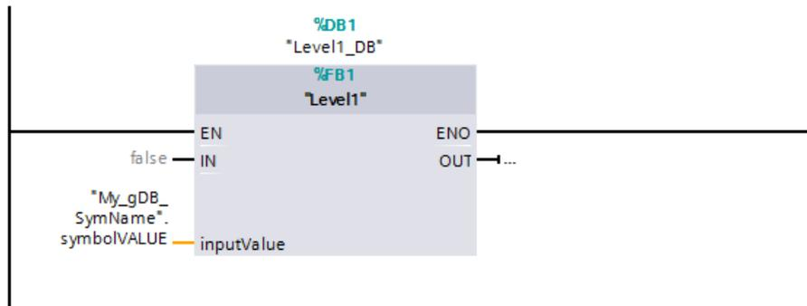
The GetSymbolName instruction is executed in the Level1 block. Input parameter inputValue of the Level1 block is examined for its interconnection using input parameter VARIABLE of the instruction. In doing so, the symbolVALUE tag is read out and output as a character string at output parameter OUT ("MySymNAME"). According to the value of input parameter SIZE, the length of the character string is limited to 60 characters.
