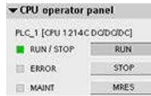
The "CPU operator panel" displays the operating mode (STOP or RUN) of the online CPU. The panel also shows whether the CPU has an error or if values are being forced.
