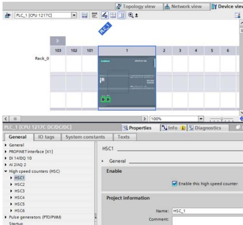
After enabling the HSC, STEP 7 sets single phase counting as the default configuration. Once you set the digital input filter for the HSC clock generator input, the program can be downloaded to the PLC, and the CPU is ready to count. To change the HSC's configuration, proceed to the next section, "Type of Counting".
