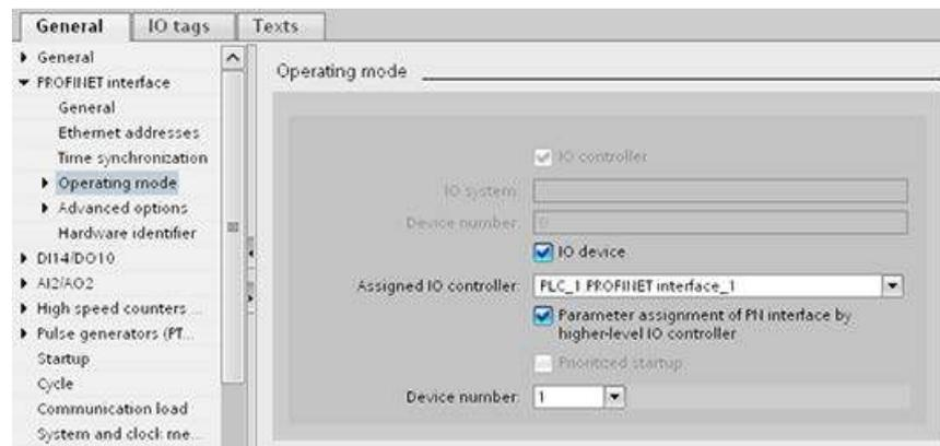
6. With the "Parameter assignment of PN interface by higher-level IO controller" check box, you specify whether the interface parameters will be assigned by the I-device itself or by a higher-level IO controller.
