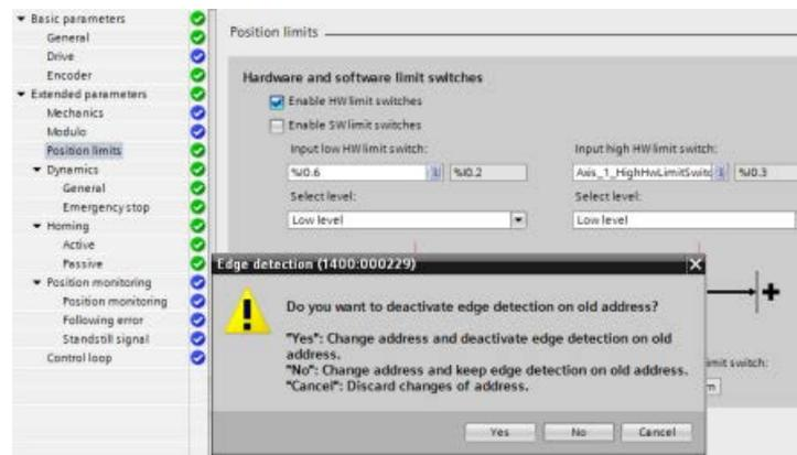
3. The "Input low HW limit switch" remains configured to I0.2 and edge detection on I0.2 remains activated:
