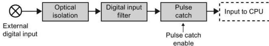
The figure below shows the response of an enabled pulse catch function to various input conditions. If you have more than one pulse in a given scan, only the first pulse is read. If you have multiple pulses in a given scan, you should use the rising/falling edge interrupt events:
