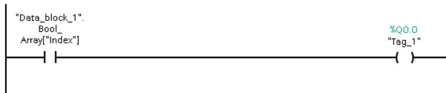
The logic with the variable array index is equivalent to the former method using the FieldRead instruction:
