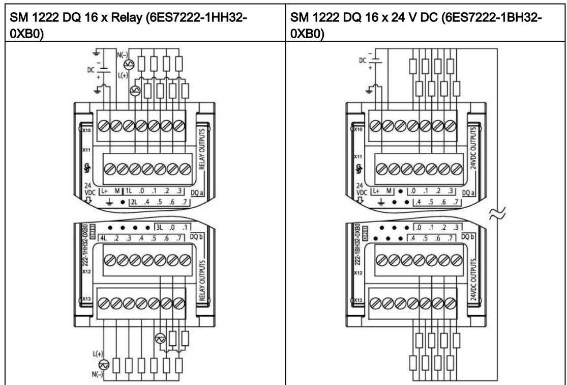
Table A- 121 Connector pin locations for SM 1222 DQ 16 x Relay (6ES7222-1HH32-0XB0)
