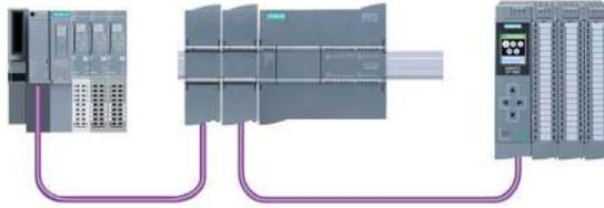
As of V3.0, you can configure a maximum of three PROFIBUS CMs per station, in which there can be any combination of DP master or DP slave CMs. DP masters in a V3.0 or greater CPU firmware implementation can each control a maximum of 32 slaves.
