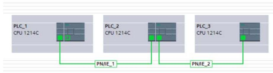
In order to check routing from either S7 subnet to the other S7 subnet, PLC\_1 must establish a transport connection to PLC\_3, and PLC\_3 must establish a connection to PLC\_1. Doing so, makes sure that routing from the PLC's PN/IE interface to a CP module is possible as well as routing from a CP module to the PLC's PN/IE interface.
