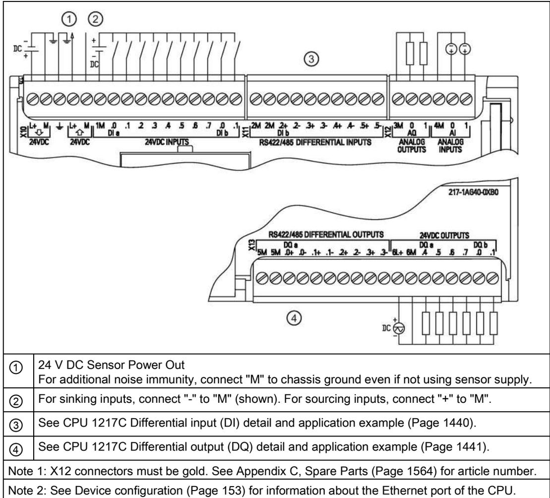
Table A- 105 Connector pin locations for CPU 1217C DC/DC/DC (6ES7217-1AG40-0XB0)
