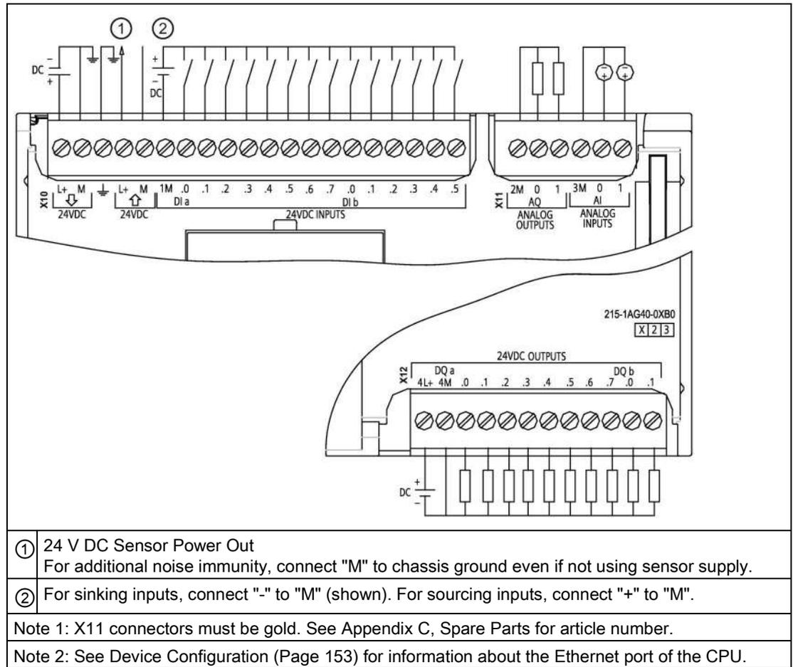
Table A- 86 Connector pin locations for CPU 1215C DC/DC/DC (6ES7215-1AG40-0XB0)
