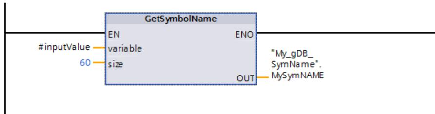
Interconnect the inputValue parameter of the Level1 block as follows.
