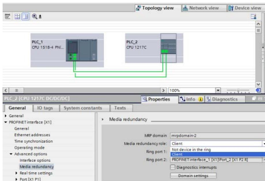
4. Under "Media redundancy role", assign the "Manager (Auto)", "Client", or "Not device in the ring" role to the device.
