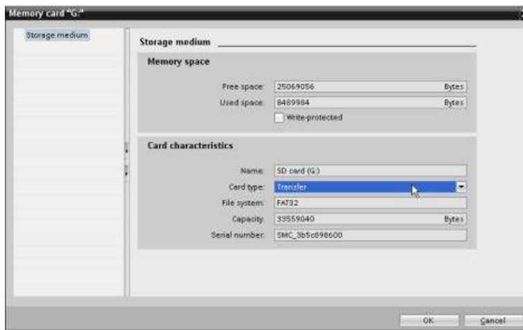
5. Add the program by selecting the CPU device (such as PLC\_1 [CPU 1214C DC/DC/DC]) in the Project tree and dragging the CPU device to the memory card. (Another method is to copy the CPU device and paste it to the memory card.) Copying the CPU device to the memory card opens the "Load preview" dialog.
