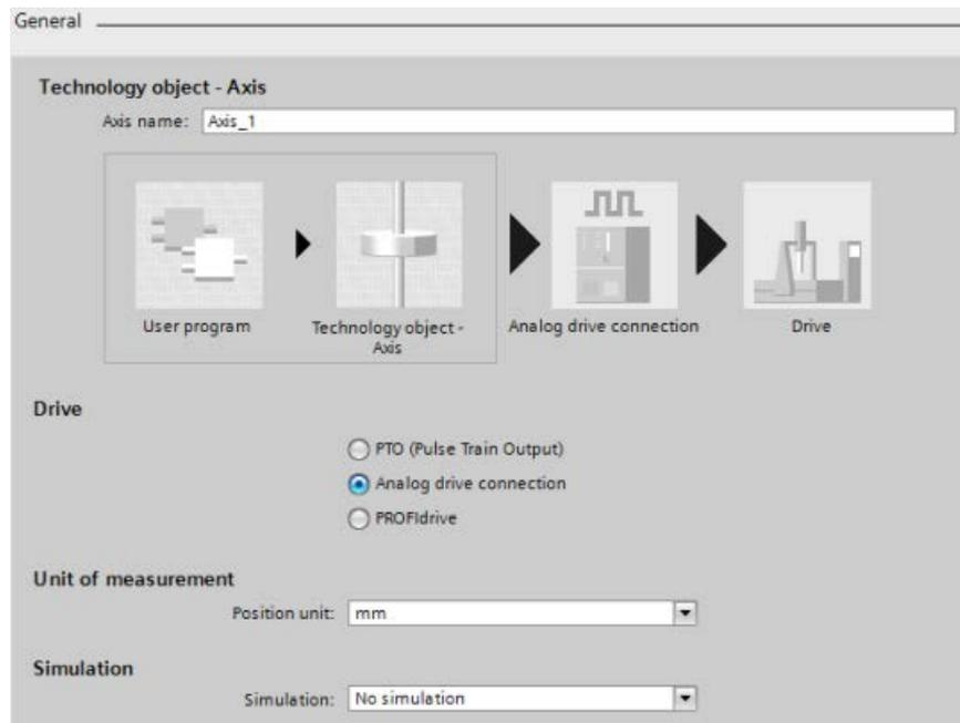
3. You now need analog outputs and a drive enable for your drive configuration. Go to the Device View of the ET 200SP interface module and the Device Overview entry for the TM Pulse module. Using the starting Q address for the TM Pulse module and the Control interface and Feedback interface tables in the *SIMATIC ET 200SP Technology module TM Pulse 2x24V (6ES7138-6DB00-0BB1) Manual*, you can determine the following analog outputs and drive enable required for your drive:
