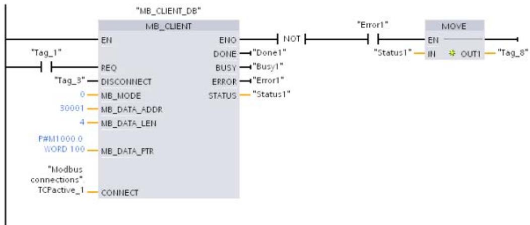
**Network 2:** Modbus function 3 - Read holding register words from a Modbus TCP server
