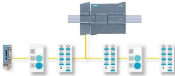
To use AS-i with S7-1200 V4.0 CPUs, you must upgrade the AS-i Master CM firmware to V1.1.
