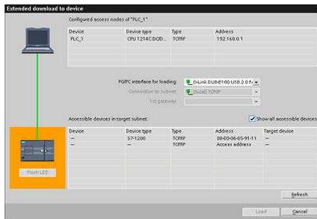
Use the CPU "Download to device" function and the "Extended download to device" dialog to show all accessible network devices and ensure that unique IP addresses have been assigned to all devices. This dialog displays all accessible and available devices with their assigned MAC or IP addresses. MAC addresses are all-important in identifying devices that are missing the required unique IP address.
