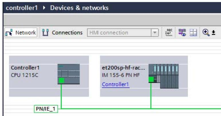
6. Double-click the IO device and insert all required modules and submodules from the hardware catalog in the device overview table.
