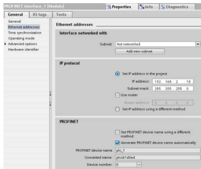
**IP addresses properties:** In the Properties window, select the "Ethernet addresses" configuration entry. STEP 7 displays the Ethernet address configuration dialog, which associates the software project with the IP address of the CPU that will receive that project.
