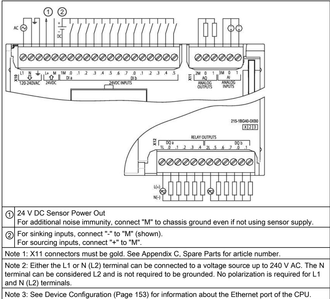
Table A- 82 Connector pin locations for CPU 1215C AC/DC/Relay (6ES7215-1BG40-0XB0)
