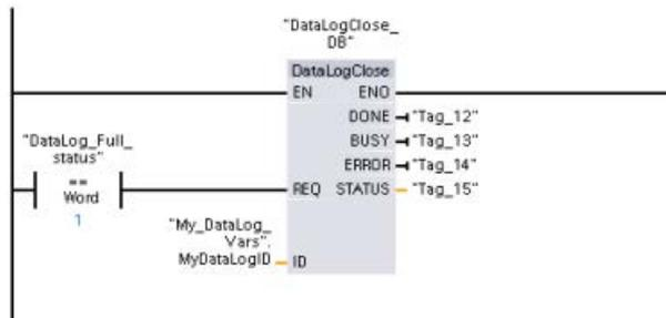
**Network 7** A positive signal edge DataLogOpen REQ input simulates the user pushing a button on an HMI that opens a data log file. If you open a Data log file that has all records filled with process data, then the next DataLogWrite operation will overwrite the oldest record. You may want to preserve the old Data log and instead create a new data log, as shown in network 7.
