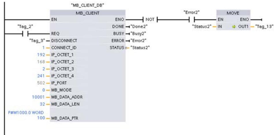
**13.8.4.3 Example: Legacy MB\_CLIENT 2: Multiple requests with different TCP connections**
