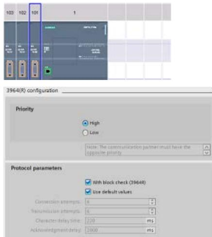
The "Properties" tab of the inspector window displays the parameters of the selected CM. Select "3964(R) configuration" to edit the following parameters:
