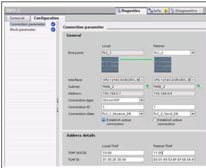
For the TCP, ISO-on-TCP, and UDP Ethernet protocols, use the "Properties" of the instruction (TSEND\_C, TRCV\_C, or TCON) to configure the "Local/Partner" connections.
