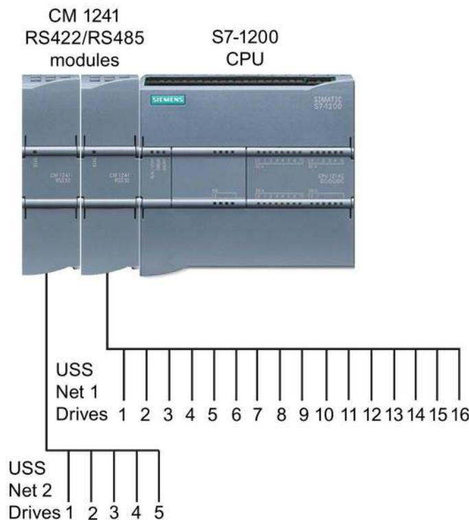
Prior to the release of STEP 7 V13 SP1 and the S7-1200 V4.1 CPUs, the USS communication instructions existed with different names, and in some cases, slightly different interfaces. The general concepts apply to both sets of instructions. Refer to the individual legacy USS instructions for programming information.
