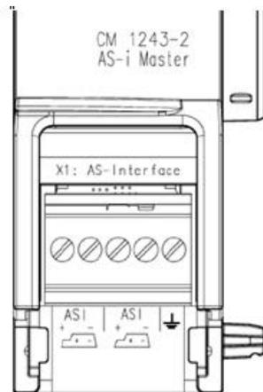
If the AS-i shaped cable is used, you can recognize the correct polarity of the cable by means of the symbol
