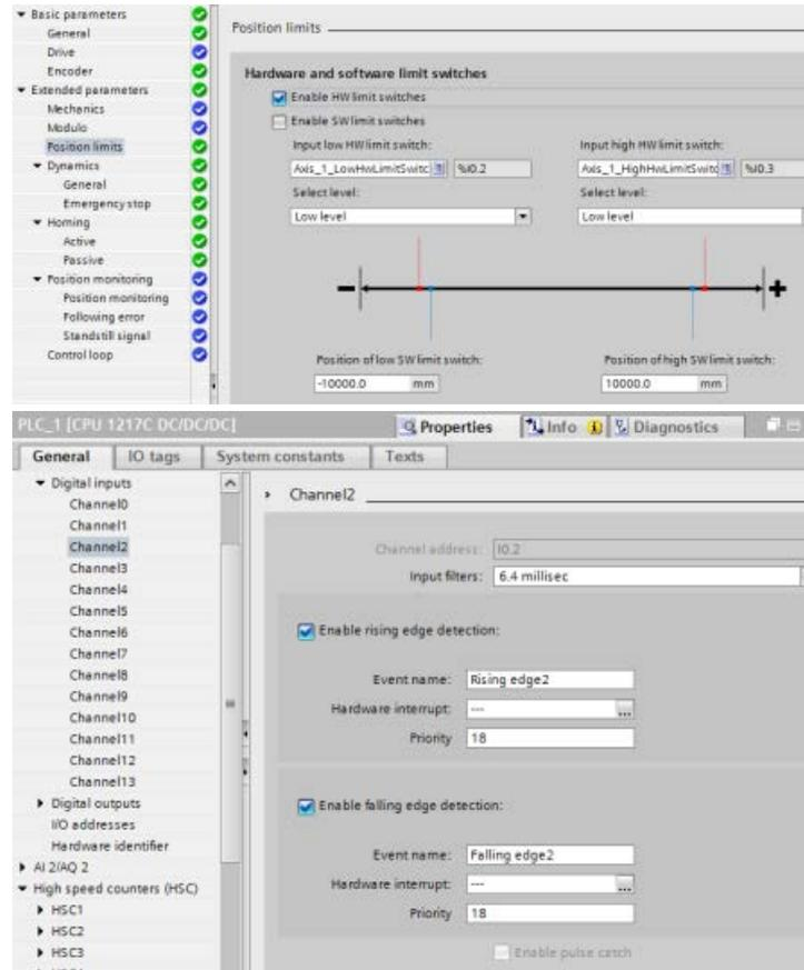
2. You change "Input low HW limit switch" to I0.6 and confirm. The edge detection dialog displays. You select: "Cancel".:
