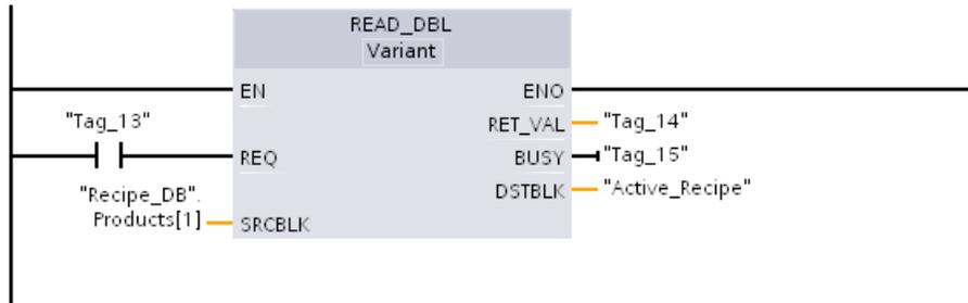
**Network 6** During run time, An HMI device could modify a component value stored in the Active\_Recipe DB. Improved recipe data can be stored by executing WRIT\_DBL. In the example, all Recipe\_DB start values for the single recipe "Recipe\_DB". Products[1] are overwritten by the current values from the "Active\_Recipe" DB.
