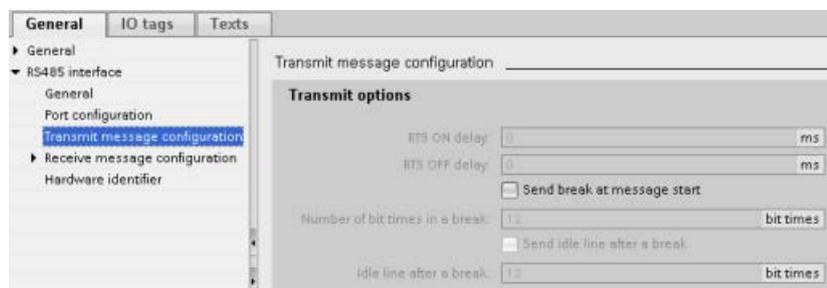
You can also dynamically configure or change the transmit message parameters from the user program by using the Send\_Config (Page 1112) instruction.
