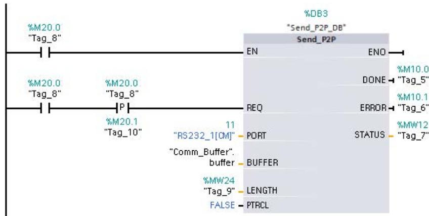
**Network 4:** monitor the DONE output of SEND\_PTP and reset the transmit flag (Tag\_8 at M20.0) when the transmit operation is complete. When the transmit flag is reset, the RCV\_PTP instruction in Network 1 is enabled to receive the next message.
