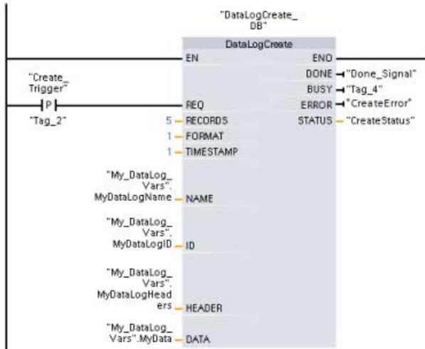
**Network 2** Capture the DONE output from DataLogCreate because it is only valid for one scan.
