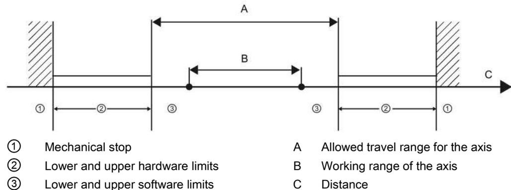
Hardware and software limit switches must be activated prior to use in the configuration or in the user program. Software limit switches are only active after homing the axis.
