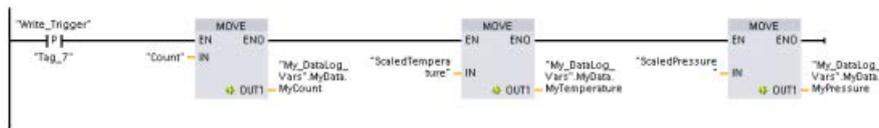
**Network 5** The EN input state is based upon when the DataLogCreate operation is complete. A create operation extends over many scan cycles and must be complete before executing a write operation. The positive edge signal on the REQ input is the event that triggers an enabled write operation.
