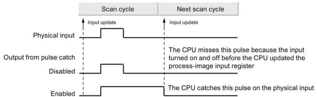
Because the pulse catch function operates on the input after it passes through the input filter, you must adjust the input filter time so that the pulse is not removed by the filter. The figure below shows a block diagram of the digital input circuit:
