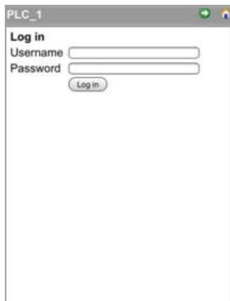
The log in frame is near the upper left corner on each standard Web page when displayed from a PC or a wide mobile device.
