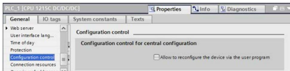
4. Create a PLC data type to contain the control data record. Configure it as a struct that includes four USInts for configuration control information and additional USInts that correspond to the slots of a maximum S7-1200 device configuration, as follows:
