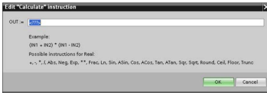
For this example, enter the following equation for scaling a raw analog value. (The "In" and "Out" designations correspond to the parameters of the Calculate instruction.)
