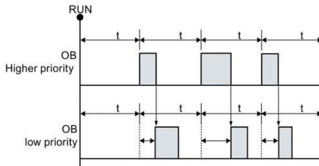
If you want to start the execution of a lower priority OB on a fixed time cycle, then phase shift time should be greater than the processing time of higher priority OBs.
