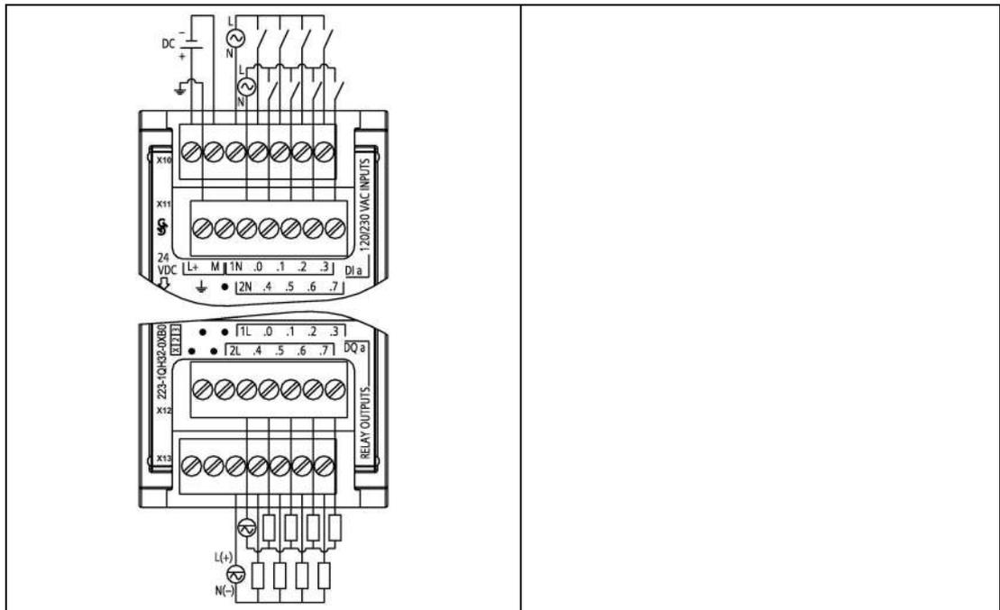
Table A- 136 Connector Pin Locations for SM 1223 DI 8 x 120/240 V AC, DQ 8 x Relay (6ES7223-1QH32-0XB0)
