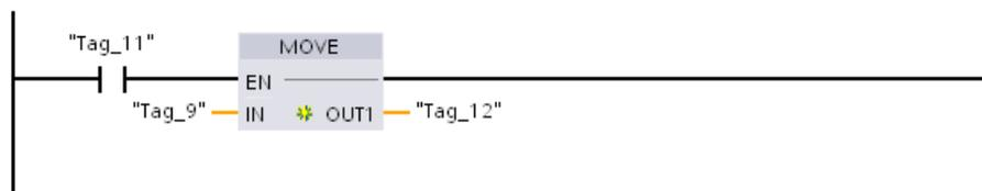
**Network 5** READ\_DBL copies the start values from one recipe "Recipe\_DB". Products[1] (in CPU load memory) to the Active\_Recipe DB current values (in CPU work memory). After READ\_DBL execution, your program logic can access the recipe component values by addressing locations in the Active\_Recipe DB. For example, the symbolic addresses ( "Active\_Recipe".productname) and ("Active\_Recipe.water) provide your program logic with the current recipe name and quantity of water.
