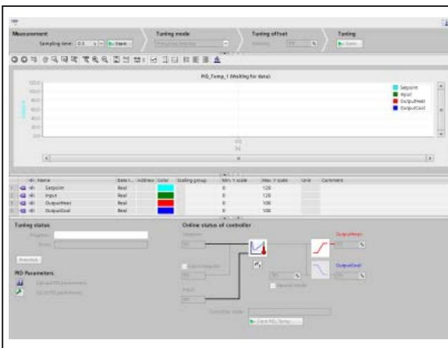
**Measurement:** To display the setpoint, the process value (input value) and the output value in a real-time trend, enter the sample time and click the "Start" button.
