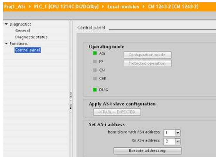
In the "Set AS-i address" field, you can change the AS-i slave address. A new slave that has not been assigned an address always has address 0. It is detected by the master as a new slave without an address assignment and is not included in normal communication until assigned an address.
