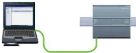
Programming device connected to the CPU
