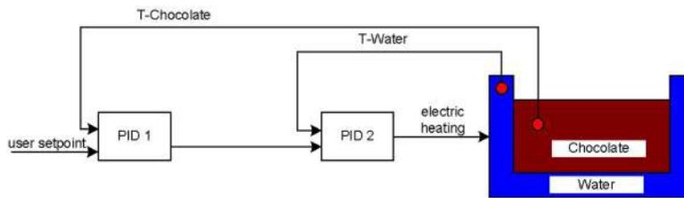
Figure 10-7 PID\_Temp\_Cascade\_Operation\_Block\_Diagram
