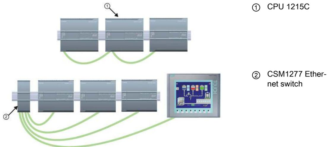
The CPU 1215C and the CPU 1217C have a built-in 2-port Ethernet switch. You can have a network with a CPU 1215C and two other S7-1200 CPUs. You can also use the rack-mounted CSM1277 4-port Ethernet switch for connecting multiple CPUs and HMI devices.
