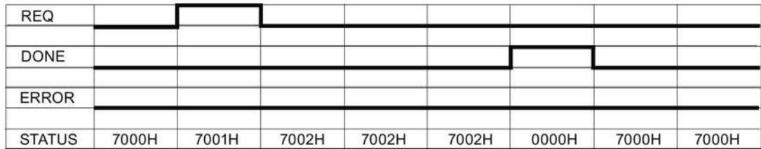
The following diagram shows the relationship of DONE, ERROR and STATUS parameters when there is an error.
