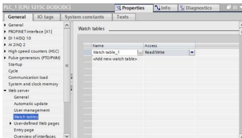
After you complete the watch table configuration in the Web server section of the device configuration, download your hardware configuration to the CPU.
