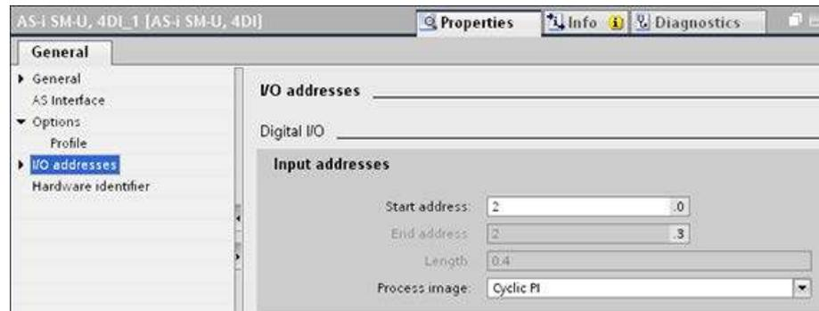
You can access the data of the AS-i slaves in the user program by using their I/O addresses with the appropriate bit logic operations (for example, "AND") or bit assignments. The following simple program illustrates how the assignment works:
