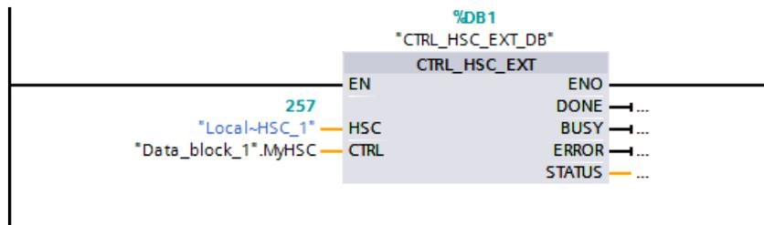
After you configure the HSC in the PLC, you can execute the `CTRL_HSC_EXT` instruction. If an error occurs, `ENO` is set to "0" and the `STATUS` output indicates the condition code.
