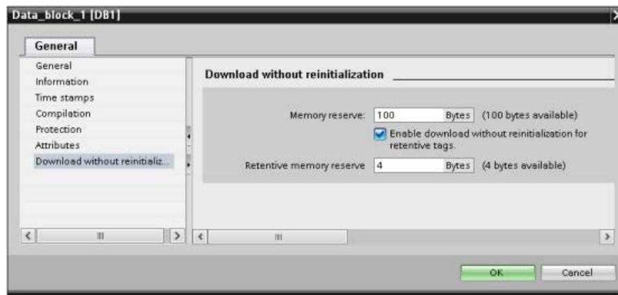
The "Download without reinitialization" feature allows you to extend a data block by adding more data block tags and download the extended data block in RUN mode. In this way, you can add tags to a data block and download it without reinitializing your program. The CPU retains the values of the existing data block tags and initializes the newly-added tags to their start values.
