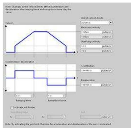
**Dynamics:** You can configure the motion dynamics and the behavior of the emergency stop command.
