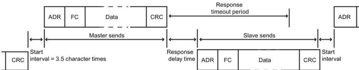
The response timeout period RESP\_TO is the amount of time a Modbus master waits for the start of a response from a Modbus slave. This time period is not defined by the Modbus protocol, but is a parameter of each Modbus master. The frequency of execution (the time between one execution and the next execution) of MB\_SLAVE must be based on the particular parameters of your Modbus master. At a minimum, you should execute MB\_SLAVE twice within the response timeout period of the Modbus master.
