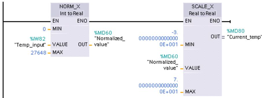
Note that if the analog input was from an analog signal module or signal board using voltage, the MIN value for the NORM\_X instruction would be -27648 instead of 0.
