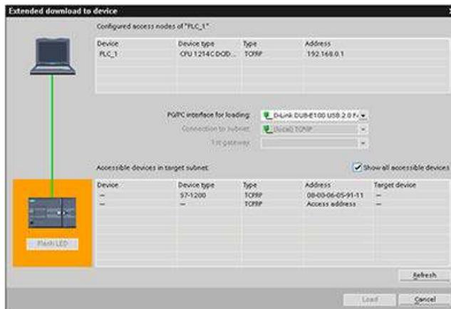
If the required network device is not in this list, communications to that device have been interrupted for some reason. The device and network must be investigated for hardware and/or configuration errors.
