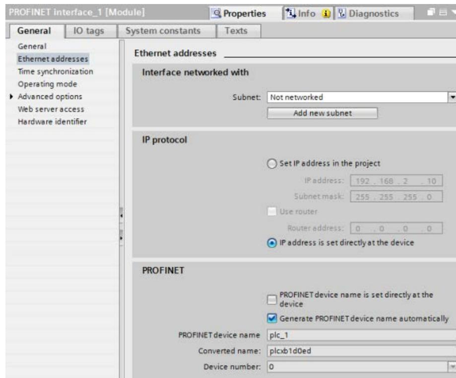
**Example: Using the T\_CONFIG instruction to change IP parameters and PROFINET IO device names**
