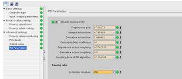
You can now change the value of any of your PID controller configuration parameters as shown in the figure below.
