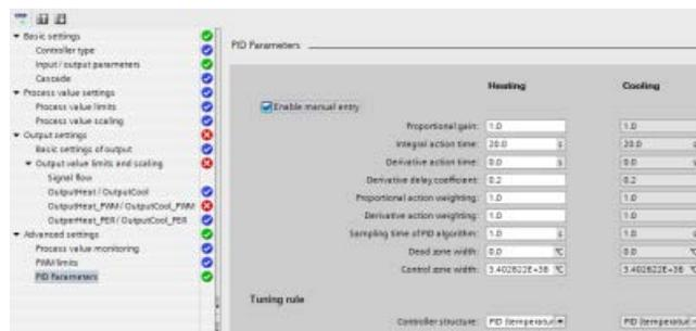
You can now change the value of any of your PID controller configuration parameters as shown in the figure below.
