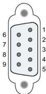
Table A- 242 Pinout of the D-sub socket
