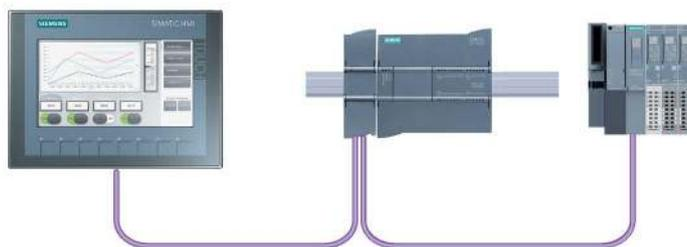
If a CM 1242-5 and a CM 1243-5 are installed together, an S7-1200 can perform as both a slave of a higher-level DP master system and a master of a lower-level DP slave system, simultaneously:
