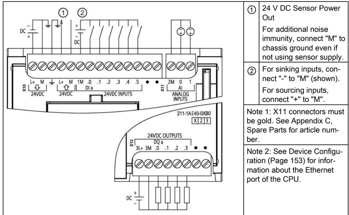
Table A- 27 Connector pin locations for CPU 1211C DC/DC/DC (6ES7211-1AE40-0XB0)
