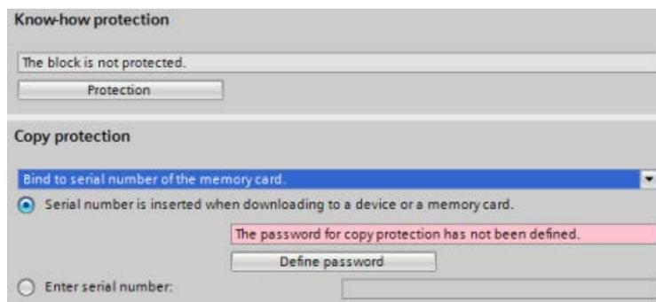
3. For binding to the serial number of a CPU or memory card, select either to insert the serial number when downloading, or enter the serial number for the memory card or CPU.
