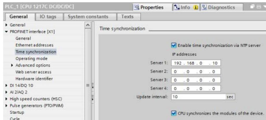
By default, neither time synchronization using the NTP server nor time synchronization of the CP clocks to the CPU's clock is enabled.
