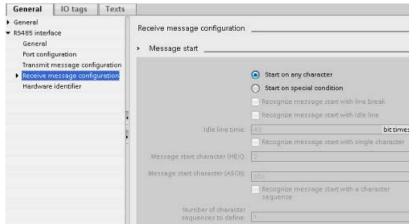
You can also dynamically configure or change the receive message parameters from the user program by using the `Receive_Config` instruction (Page 1115).
