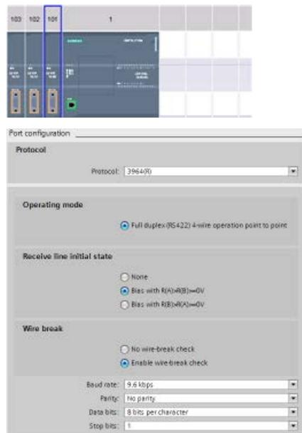
The "Properties" tab of the inspector window displays the parameters of the selected CM. Select "Port configuration" to edit the following parameters:
