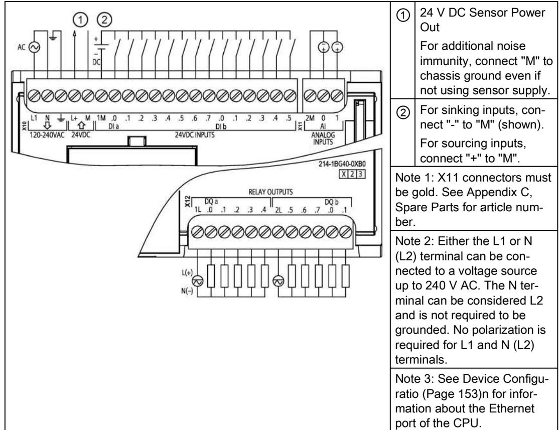
Table A- 61 Connector pin locations for CPU 1214C AC/DC/Relay (6ES7214-1BG40-0XB0)
