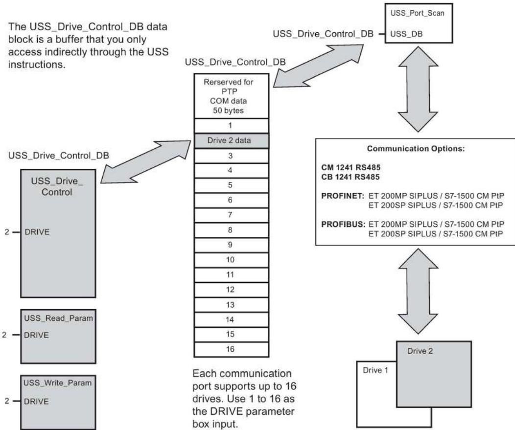
All drives (up to 16) connected to a single RS485 port are part of the same USS network. All drives connected to a different RS485 port are part of a different USS network. Each USS network is managed using a unique data block. All instructions associated with a single USS network must share this data block. This includes all USS\_Drive\_Control, USS\_Port\_Scan, USS\_Read\_Param, and USS\_Write\_Param instructions used to control all drives on a single USS network.
