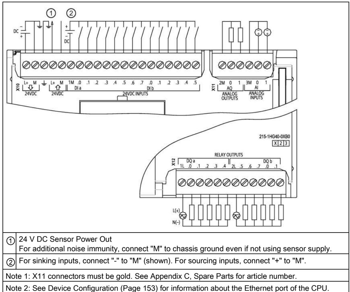
Table A- 84 Connector pin locations for CPU 1215C DC/DC/Relay (6ES7215-1HG40-0XB0)
