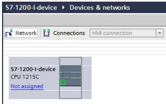
4. Double-click the IO device and configure all required modules and submodules.
