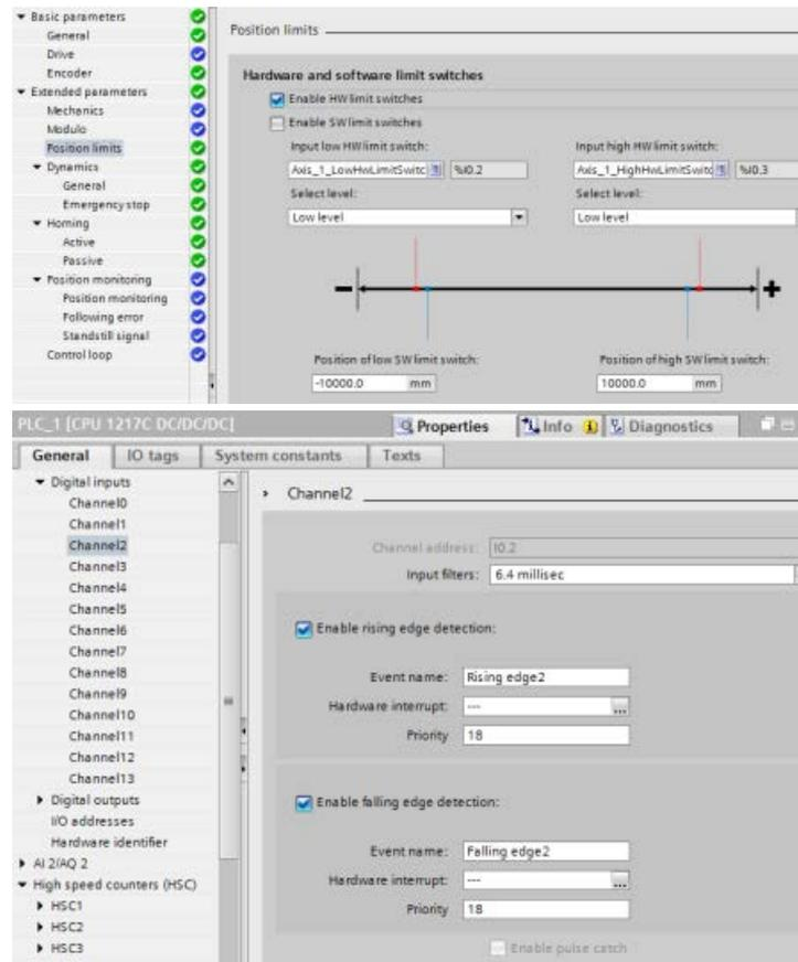
2. You change "Input low HW limit switch" to I0.6 and confirm. The edge detection dialog displays. You select: "Yes: Change address and deactivate edge detection on old address.":
