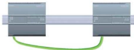
A CPU can communicate with another CPU on a network by using the TSEND\_C and TRCV\_C instructions.
