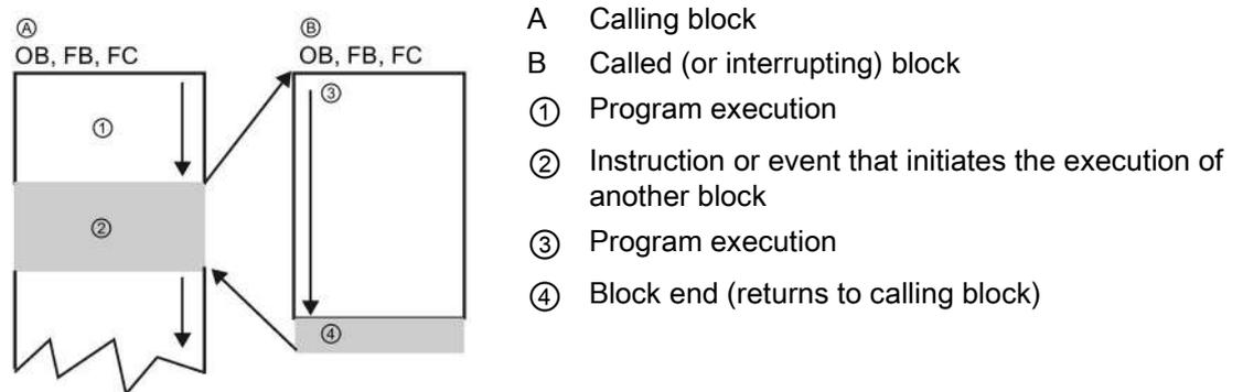
You can nest the block calls for a more modular structure. In the following example, the nesting depth is 3: the program cycle OB plus 3 layers of calls to code blocks.
