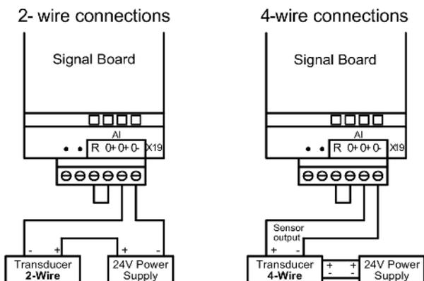
Table A- 209 Wiring diagram for the analog input SB
