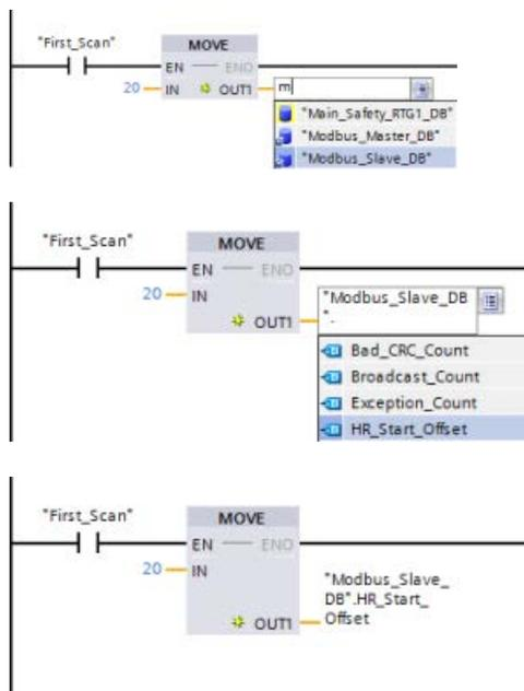
Entering a Modbus slave variable using the default DB name:
