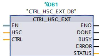
2. Attach the HSC's hardware identifier, found in the HSC's properties, to the "HSC" pin of the ladder instruction. You can also select one of the six "Hw\_Hsc" objects from the dropdown menu of this input pin. The default tag name for HSC1 is "Local~HSC\_1":
