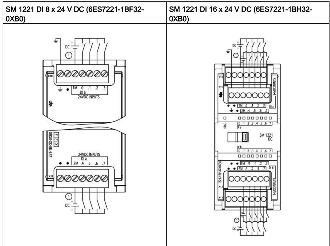
① For sinking inputs, connect "-" to "M" (shown). For sourcing inputs, connect "+" to "M".
