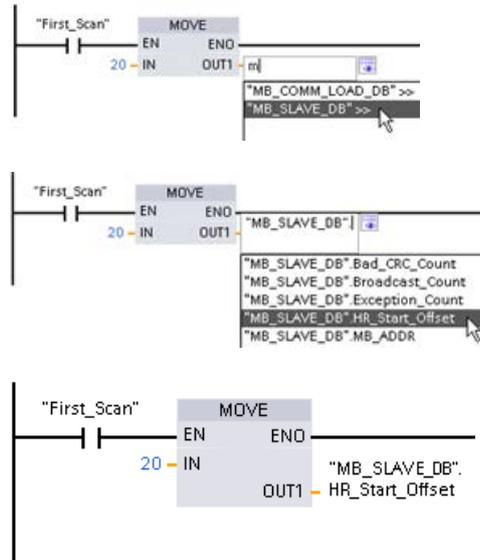
Entering a Modbus slave variable using the default DB name:
