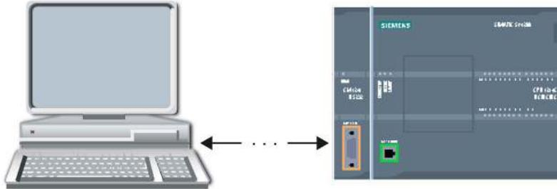
You must connect the communication interface of the CM 1241 RS232 module to the RS232 interface of the PC, which is normally COM1. Because both of these ports are Data Terminal Equipment (DTE), you must switch the receive and transmit pins (2 and 3) when connecting the two ports, which you can accomplish by either of the following methods:
