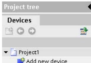
Be sure you insert the correct model and firmware version from the list. Selecting the CPU from the "Add new device" dialog creates the rack and CPU.
