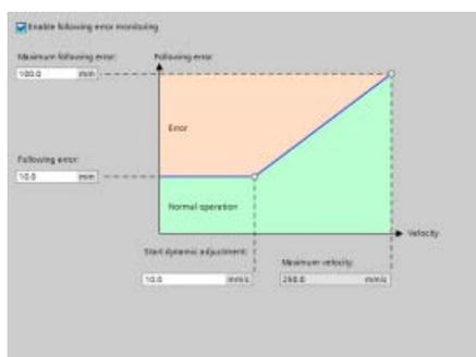
"Following error": You can configure the difference of the allowed error distance over a velocity range. You check the "Enable following error monitoring" check box to activate following error. You can configure the following parameters:
