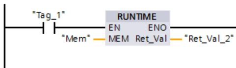
When the "Tag\_1" operand in network 1 has the signal state "1", the RUNTIME instruction executes. The starting point for the runtime measurement is set with the first call of the instruction and buffered as reference for the second call of the instruction in the "Mem" operand.
