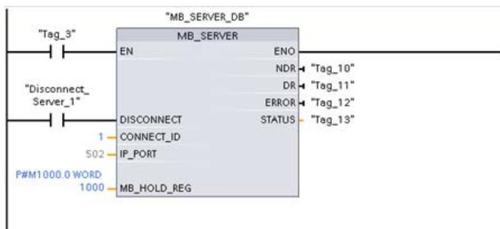
**Network 2:** Connection #2 with independent IP\_PORT, connection ID, and instance DB
