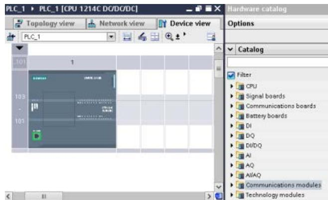
Selecting the CPU in the Device view displays the CPU properties in the inspector window.
