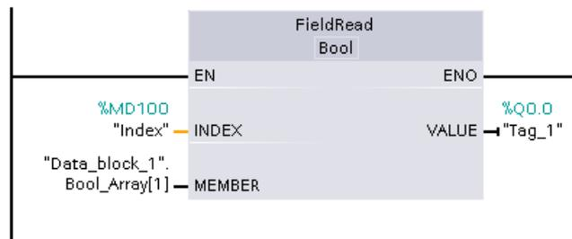
FieldWrite and FieldRead instructions can be replaced with variable array indexing logic.
