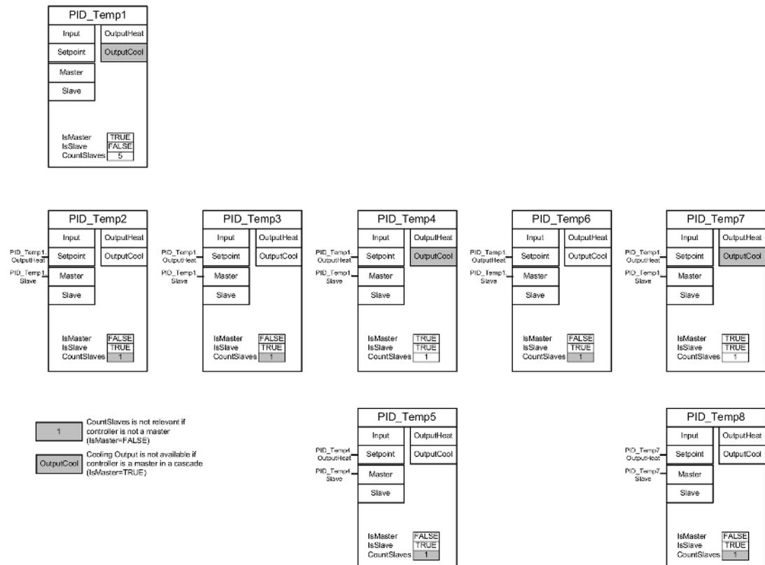
Figure 10-8 PID\_Temp\_Cascading\_communication\_connection
