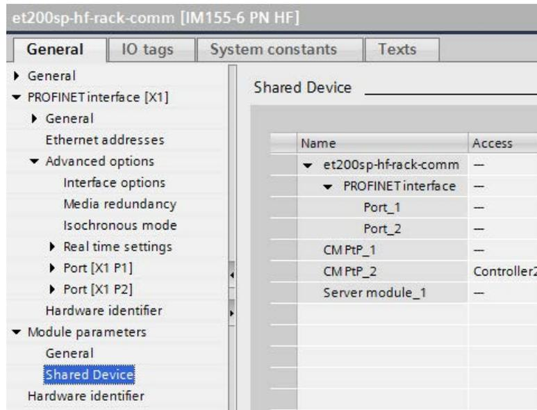
7. Finally, check whether the settings for access are "complementary" for each module or submodule in both projects. This means that if the local CPU has access in one project, the option "---" must be set in the other project and vice versa.
