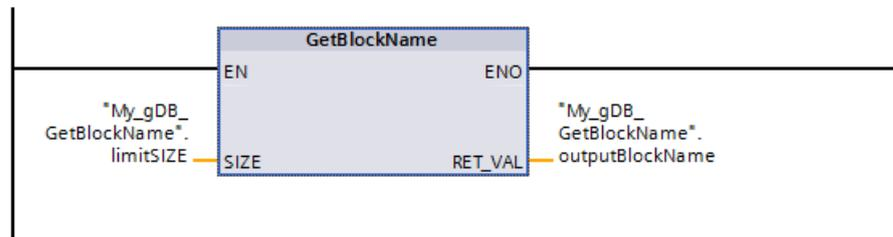
The Level1\_gbn block executes the GetBlockName instruction. GetBlockName reads out the name of the Level1\_gbn block and outputs the name as a character string at output parameter RET\_VAL(outputBlockName). Because the SIZE parameter is 0 (limitSIZE), the length of the character string is unlimited.
