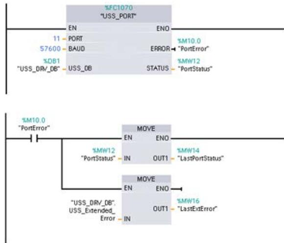
**Network 1** "PortStatus" port status and "USS\_DRV\_DB".USS\_Extended\_Error extended error code values are only valid for one program scan. The values must be captured for later processing.
