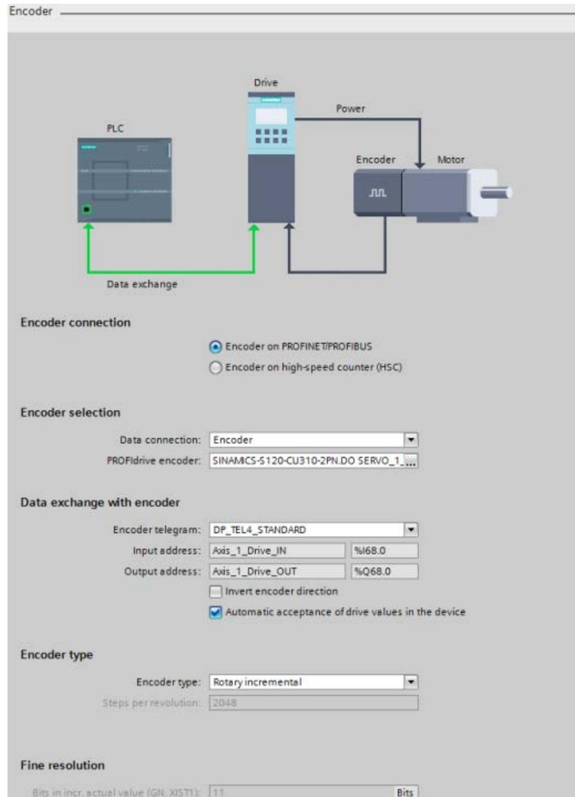
The screenshot shows the 'Encoder' configuration dialog in a software interface. At the top, a diagram illustrates the system architecture: a PLC is connected to a Drive via 'Data exchange' (green arrows). The Drive is connected to an Encoder and a Motor via 'Power' (black arrows). Below the diagram, the configuration is organized into several sections:
