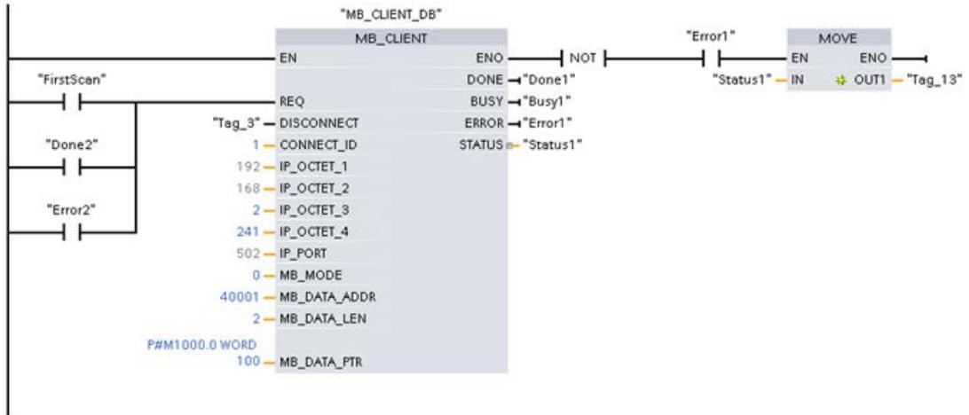
Network 2: Modbus function 3 - Read holding register words
