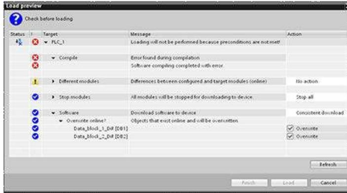
You must correct the compile error in the other block. Then, the "Load" button becomes active.
